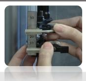
Positioning tool is used to adjust the gauge length of extensometer. It has five intervals: 10mm, 20mm, 25mm, 30mm and 50 mm
