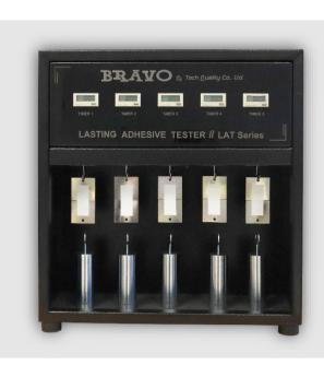
Precise room temperature shear tests are made easier with the "**BRAVO**" LAT Series Room Temperature 5 Bank Shear Tester. It performs shear tests according to PSTC-7 and ASTM D 3654 Procedure A for holding power of pressure sensitive tapes.
