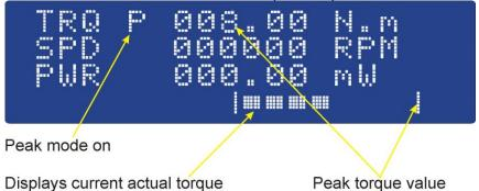
The torque bar at the bottom of the display indicates actual torque (eg: with 8 Nm peak torque value the bar indicates 4 Nm of torque applied). Note also to the right hand side that peak value is marked with a line.
