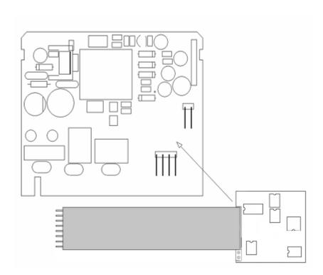
Plug the other Modbus module connector to the  $\mu400P/\mu500PT$  CPU board as shown in the figure below.
