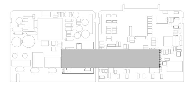
Once the Modbus module is installed, the communications are accessible from terminals 11,12 and 13 (see section 2.2).
