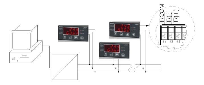
In addition, just after the last instrument in the line, a 220-Ohm termination resistance should be connected in the line between TR+ and TR-.
