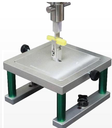
The Volodkevich Bite Jig is primarily used for shear testing on meat products although may be used for other products; it simulates a bite action similar to incisor action. Fixture width 12mm with a 1.5 radii on upper and lower fixture
