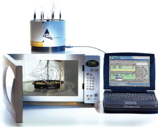
The MWS Microwave Work Station is designed to perform temperature measurements in a microwave oven equipped with a turntable. The use of fiber optic sensing technology allows complete immunity to microwave energy as well as accurate and reliable measurements inside the microwave oven cavity.
