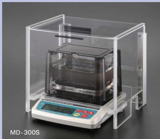
■ Indication: Weight in the air; Weight in the water; Value of specific gravity; Volume
