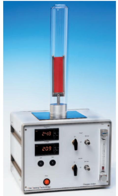
ASTM D 2863: Standard test method for measuring the minimum oxygen concentration to support candle-like combustion of plastics (oxygen index)
